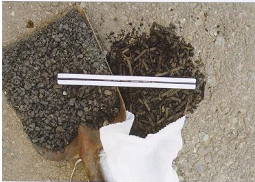
Photo 12. Erie County S.R. 4022 Shovel with Acceptable Shredded Shingles, Maximum \frac{1}{2} Inch Bag with Rejected Shingle Pieces Larger Than \frac{3}{4} Inch.
