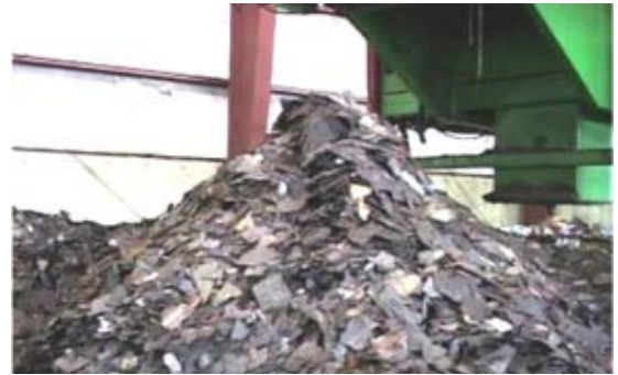
When used in the right proportions, crushed asphalt pavement and sorted asphalt shingles like these from residential roofs and sidings can be effective in asphalt pavement mixtures.
