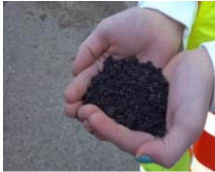
Ground up asphalt shingles can be used as a partial replacement for expensive asphalt binders in pavement mixtures.
