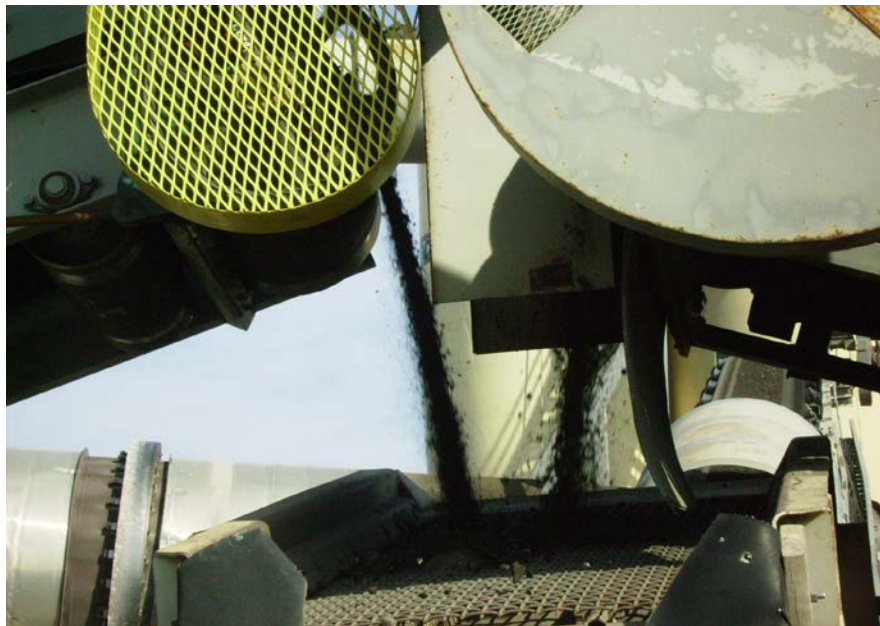
Figure 15. Vibratory Scalping Screen (after Morton, 2011).
