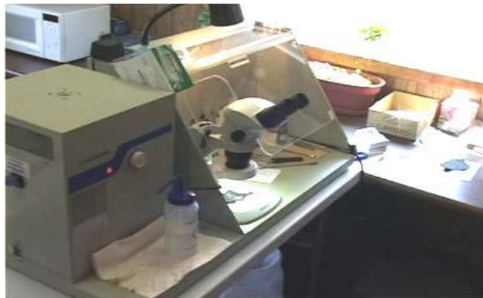
Figure 3. Setup for Asbestos Testing (after Krivit, 2007).
